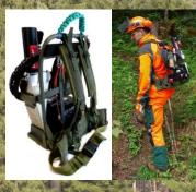
The remote-controlled StriXner battery felling system AP3 enables you to bring down a tree completely vibration free and with safety, covering a distance we to 200 metars. distance up to 80 meters!
